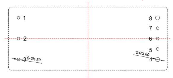
Recommended holes for PCB layout
